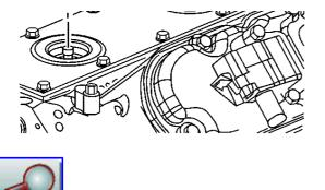
2. Remove the wiring harness assembly from the knock sensor.
